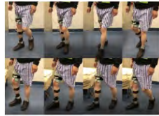
IMU-based gait phase recognition system for stroke survivors
